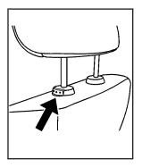
Pull the head restraint up to raise it. To lower the head restraint, press the button, located on the top of the seatback, and push the restraint down. Push down on the head restraint after the button is released to make sure that it is locked in place.
